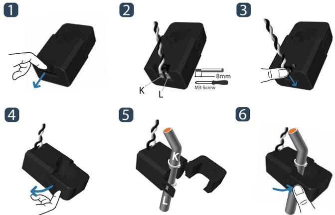
JS series of split-core current transformer offers 5A at secondary from sensed primary current for metering application. It can be used for power meter, distribution system, control panels, switchgear and other equipment. It is designed to install to live power line without disconnection as split-core compact type. Also, over-voltage protection circuit is included to offer safe, fast and cost effective installation.
