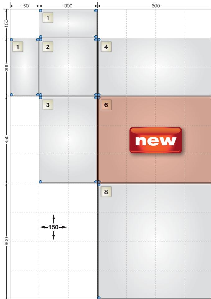
The **modular design** in a basic grid of 150 mm allows free design of the outer form. The enclosures can be combined in all directions. Obstacles at the building structure can be easily circumvented.
