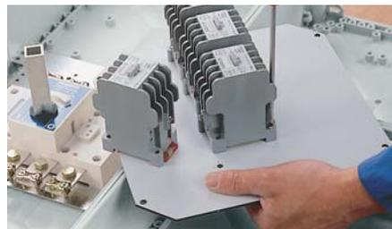
■ Equipment can be installed via mounting plates as well
